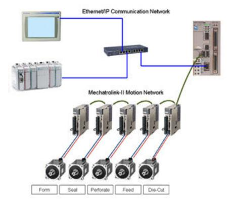
software with predefined PLCopen function blocks and user libraries saves time and speeds development for the programmer. Yaskawa's Cam Toolbox provides pre-written application code essential for Cam Generation and execution that allows easy on-the-fly changes to all cam profiles and fine-tuning of the machine cycle.
